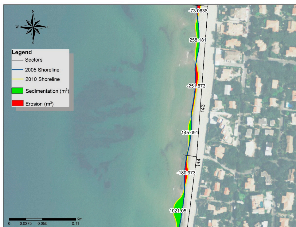
Figure 7. Shoreline comparison and extraction of aerial variation in the timeframe 2005–2010 for sector 144: Polygon extraction and aerial calculation of the erosion/sedimentation quantities are shown as positive or negative values.
