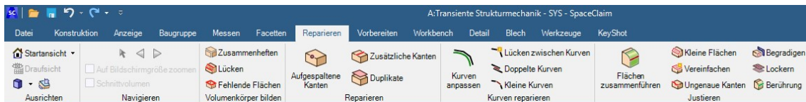
Figure 4.7: Reparation commands in SpaceClaim. Translation from German: union of faces, gaps, additional edges, missing faces and so on
