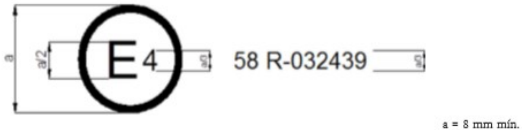
Figure 1.5: Example of a homologation mark for a vehicle approved in the Netherlands [2]
