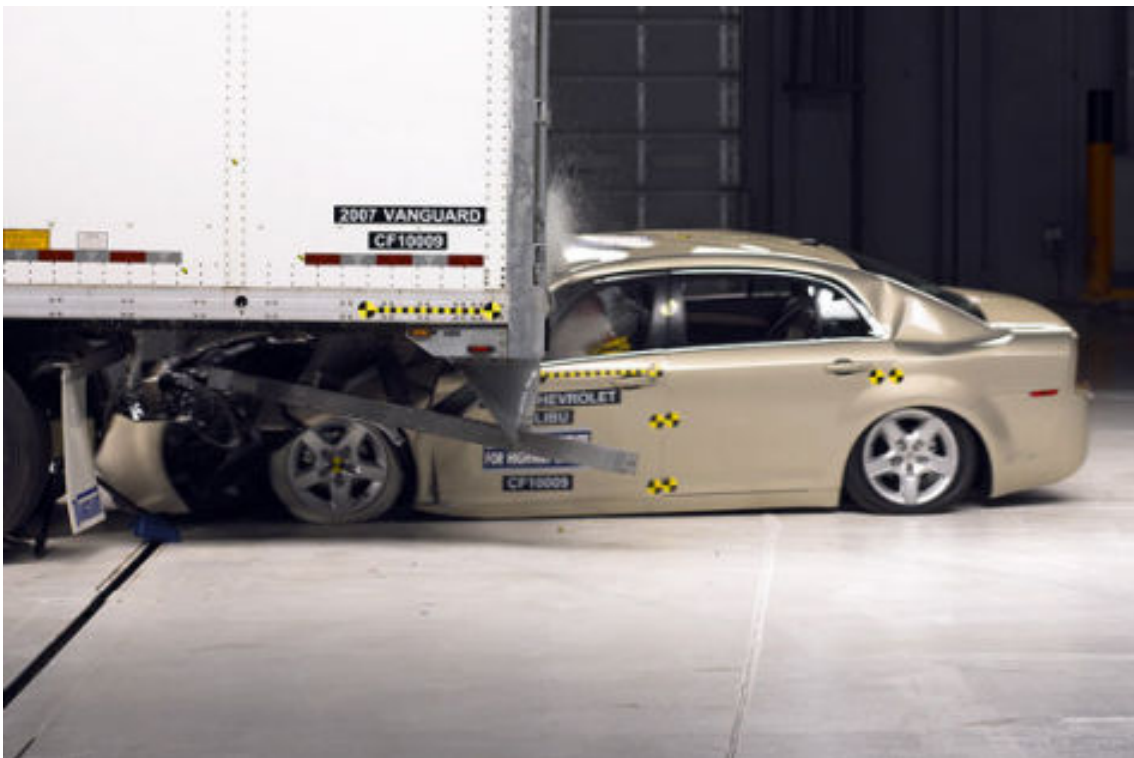
Figure 1.1: Sliding of smaller vehicle under the frame of the heavy weight vehicle [1]
