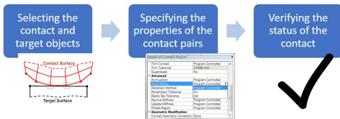
Figure 1.14: Steps and examples of contact definition in ANSYS
