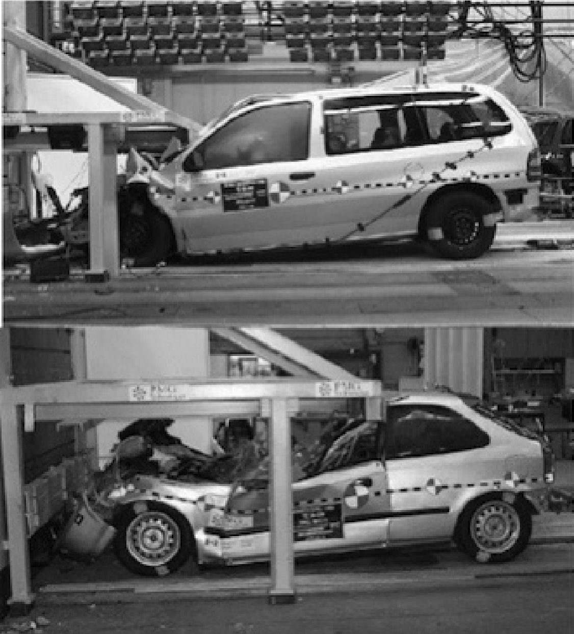
Figure 3.5: Crash tests for the same vehicle with varying collision speeds: a) 48 km/h b) 56 km/h [38]
