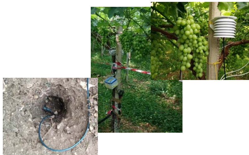
Figure 2. (A) Installation of soil moisture sensor. (B) Wireless sensor node. (C) Environmental sensor.
