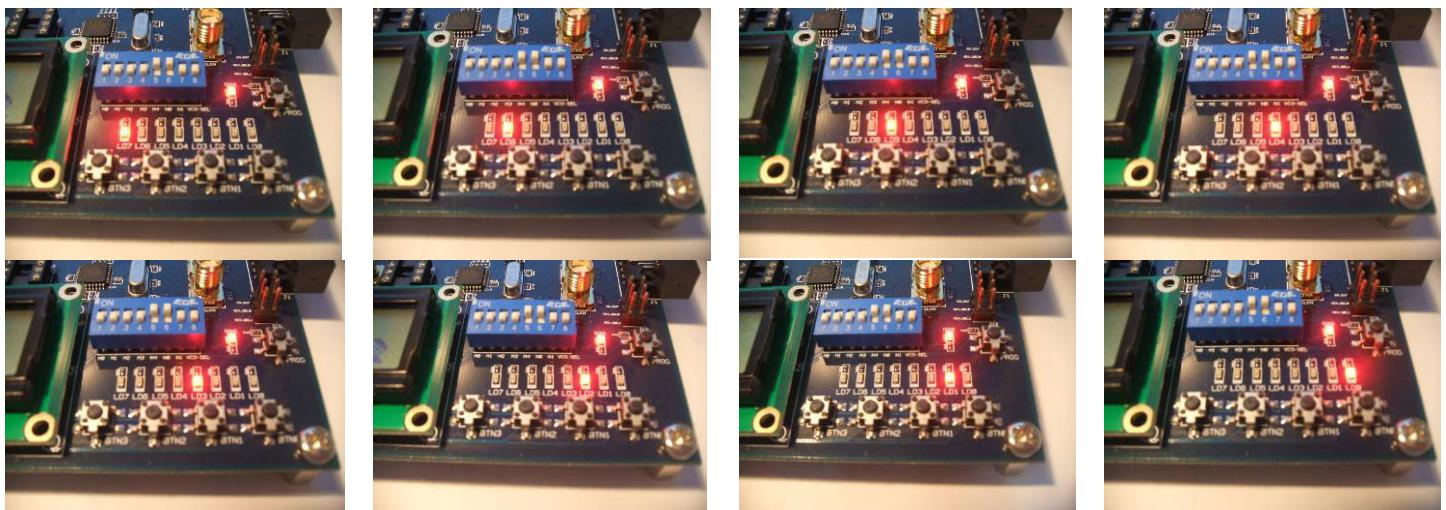
**Figura 30.** Placa Virtex-4 con *bitstream* parcial *rightshift*
