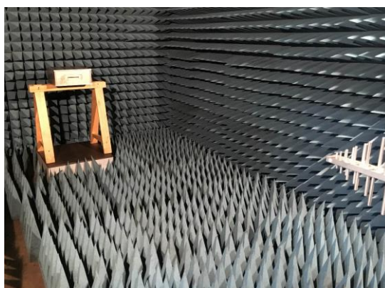
Figure 1. Shielding enclosure with an aperture in the anechoic chamber.
