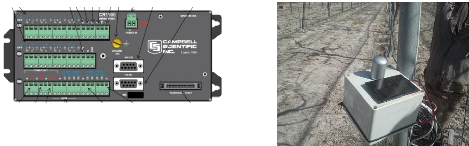
Figure 1. Campbell Scientific CR1000 Datalogger vs Wireless sensor node
