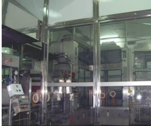
Figure 2 Ultra-clean packaging facility for fruit juices (Photo by A. López-Gómez).
