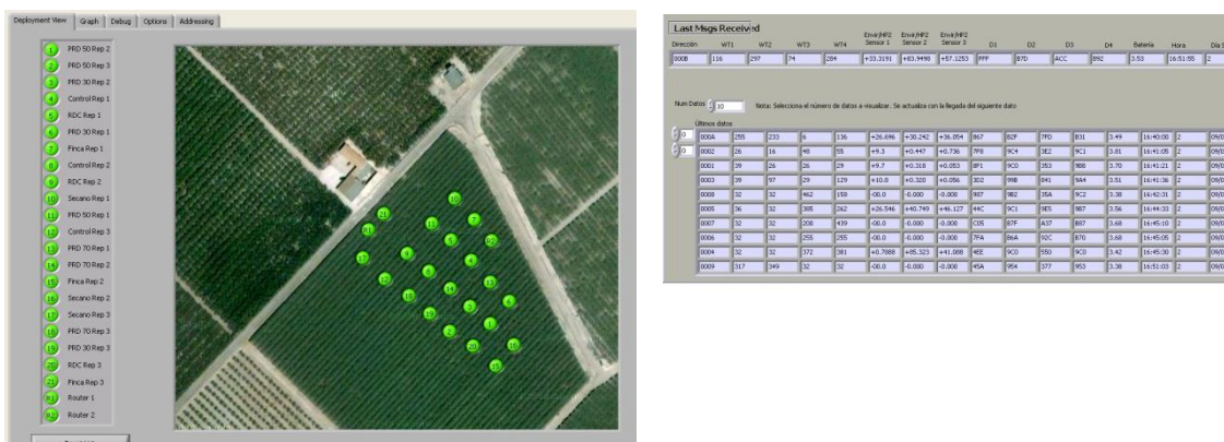
Figure 2.- WSN deployment in a wine crop. Data collected by the coordinator node.
