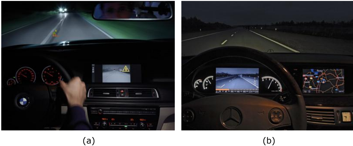
Figure 1.13: Night Vision Systems: (a) BMW far-IR Night Vision System; (b) Mercedes-Benz near-IR Night View Assist System
