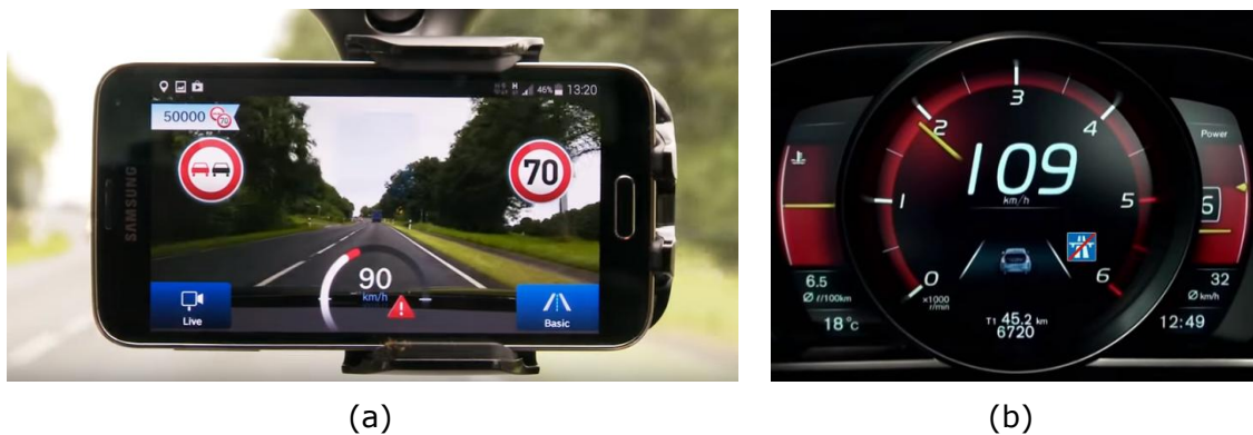
Figure 1.11: TSR Real Systems: (a) Mydriveassist real usage case; (b) Volvo V40 2012, Active TFT Traffic Signs Display
