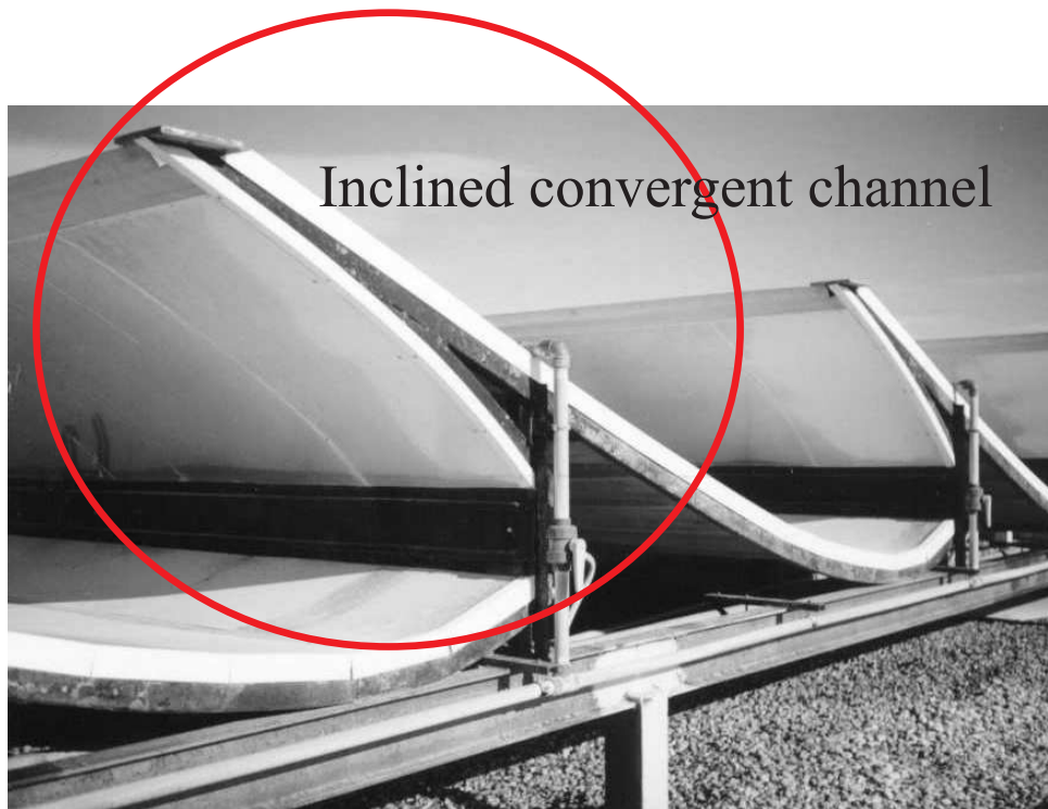
Figure 14: First experimental prototype of the hydro-solar chimney, that includes an inclined convergent channel.
