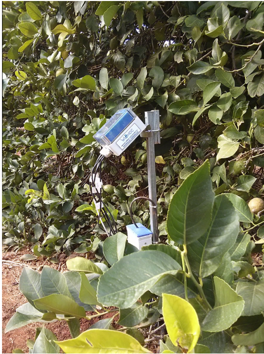
Fig. 3. Device installed in a lemon crop field.
