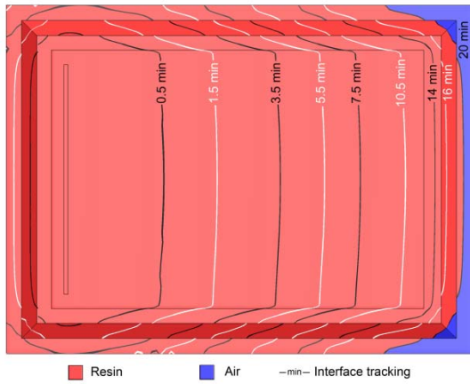
Missed Figure during revision: In-plane evolution of the resin flow front during the molding process. a) Experimental test on the distribution media (Courtesy of MTorres). b) Experimental test on the bottom ply (Courtesy of MTorres). c) Numerical results on the distribution media. a) Numerical results on the bottom ply.
