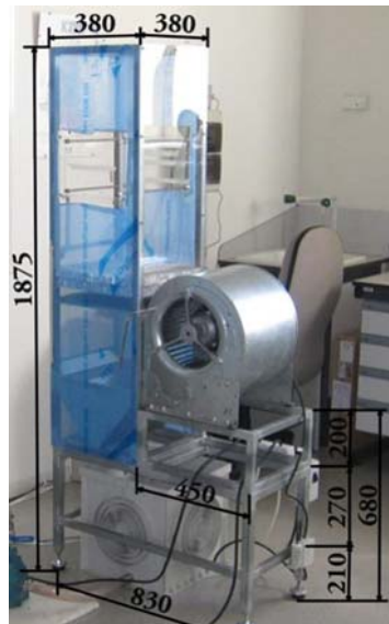
Figure 1: Experimental cooling tower.
