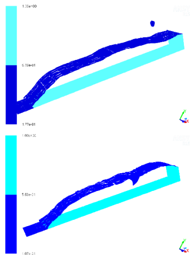
Figure 7: Droplet impact sequence. Water drop is seen in the first figure, and the groove formed
