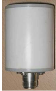
Figure B.10: Omnidirectional Electrometrics EM-6116 antenna.
