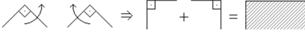
Figure 3.2: Rectangular obstacle seen as a combination of two joined wedges of interior angle \pi/2 rad.
