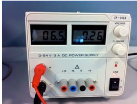
Figure B.4: Power Source EP613-A.
