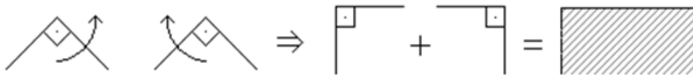
Figure C.2: Rectangular obstacle seen as a combination of two joined wedges of interior angle \pi/2 rad.
