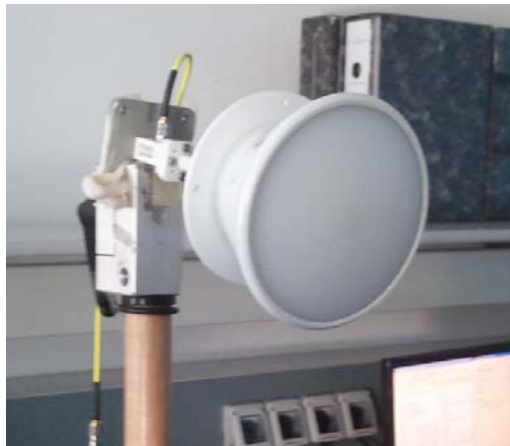
Figure B.9: Lens antenna H3445 25810-TA.
