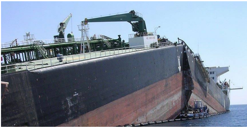
Figure 3.1.3. Collapse of the hull girder (Marineinsight.com)
