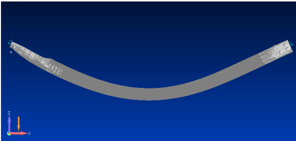
Figure 7.5.3. Numerical deflection of the vessel. Lateral view
