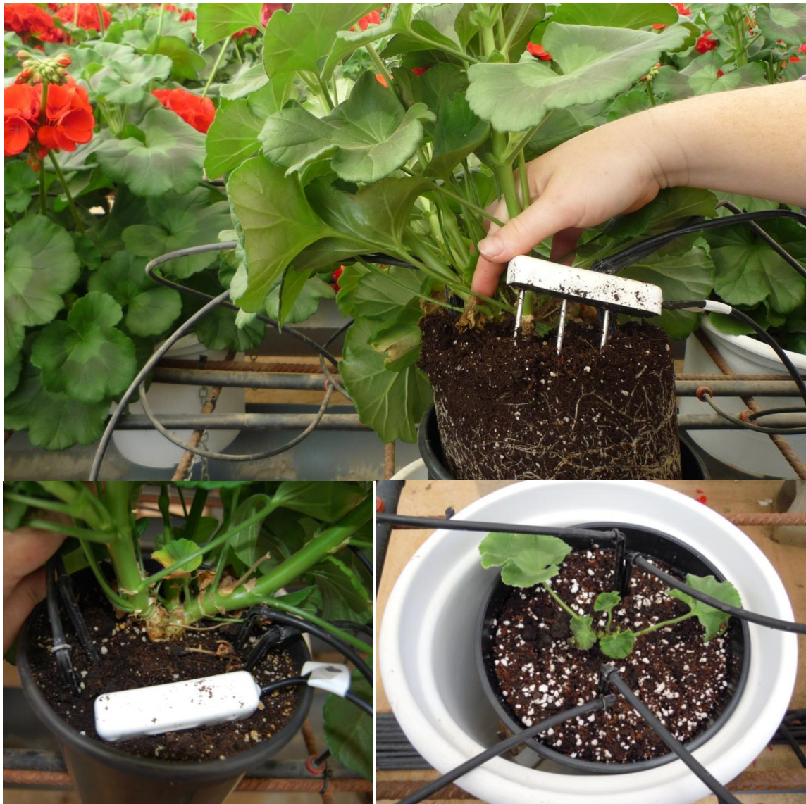
Picture 1. Details of the position of the GS3 sensor and emitters.
