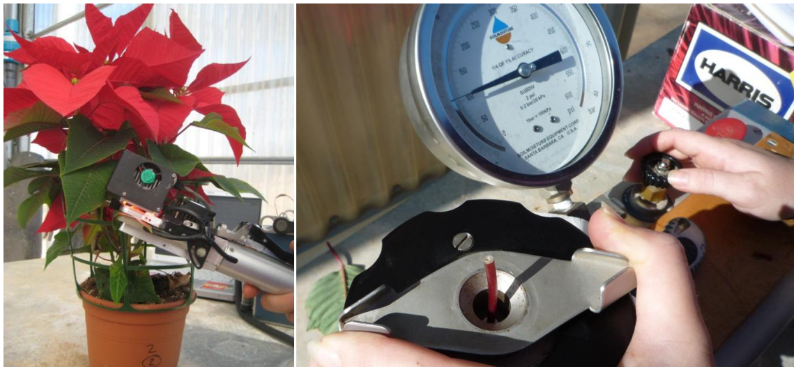
Picture 2. Details of the measurement of gas exchange and leaf water potential.
