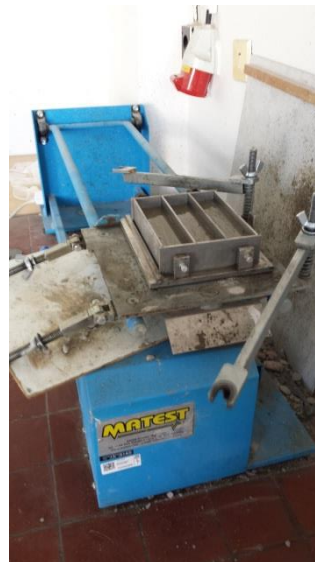
Figure 66: Cement jolting table
