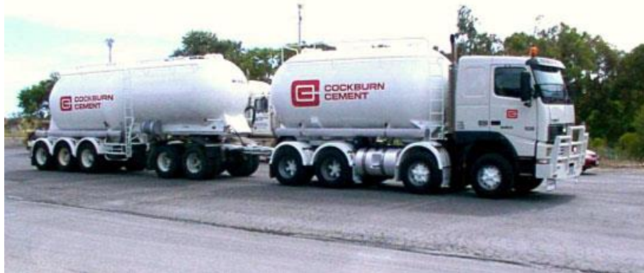
Figure 10: Bulk quantities cement transport
