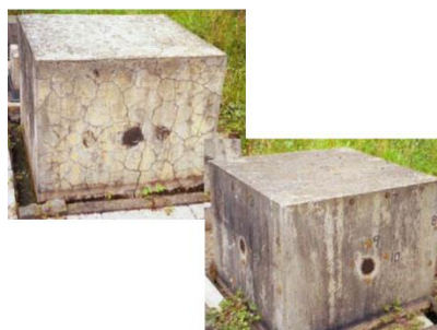
Figure 36: Concrete blocks with/without fly ash
