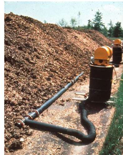
Figure 47: Aerated static piles
