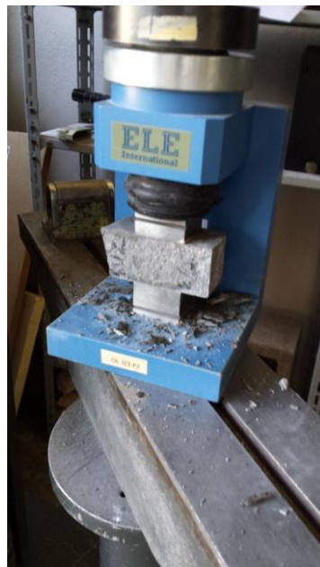
Figure 70: Compressive strength test
