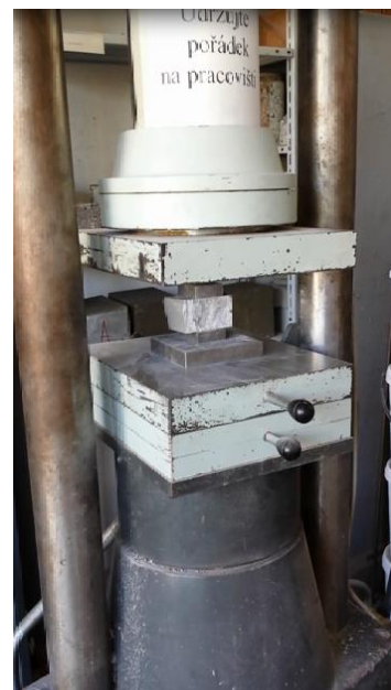
Figure 71: Compressive strength test
