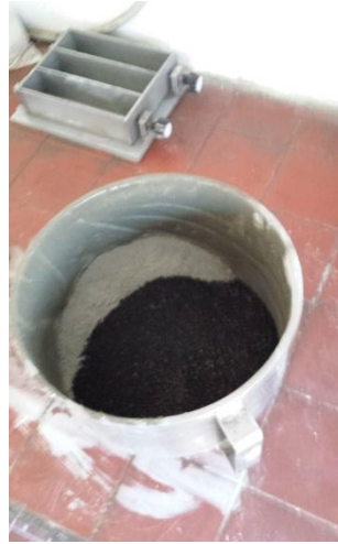
Figure 64: Mixing cement and sludge:
