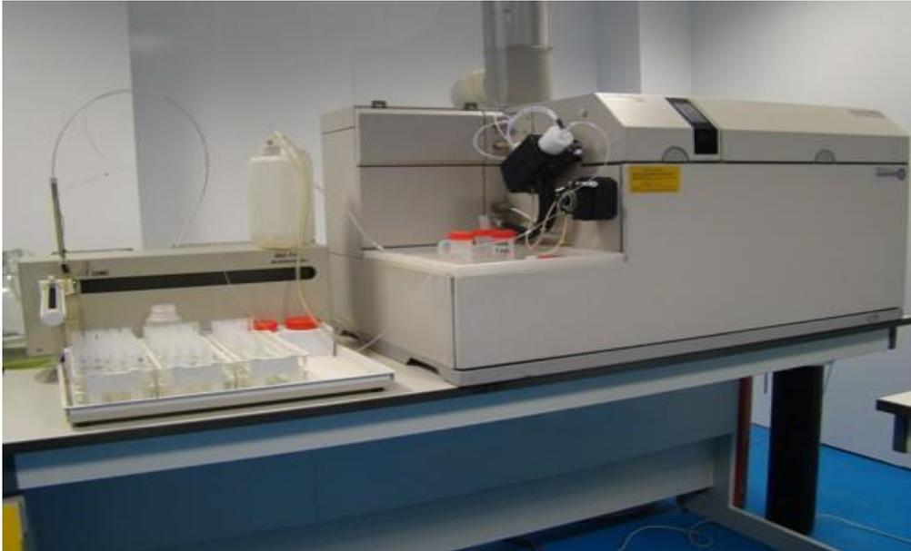
**FIGURA IV.10.-** ESPECTRÓMETRO DE MASAS CON FUENTE DE PLASMA ACOPLADO. SAIT
