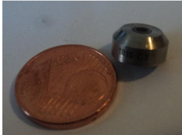
Figure 43: Water nozzle. Diameter is 0.15mm.
