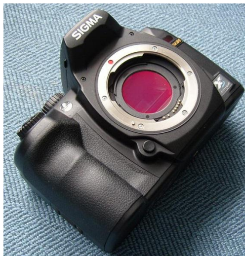
Figure 17: Example of a camera for IR photography Sigma - SD14 [24].
