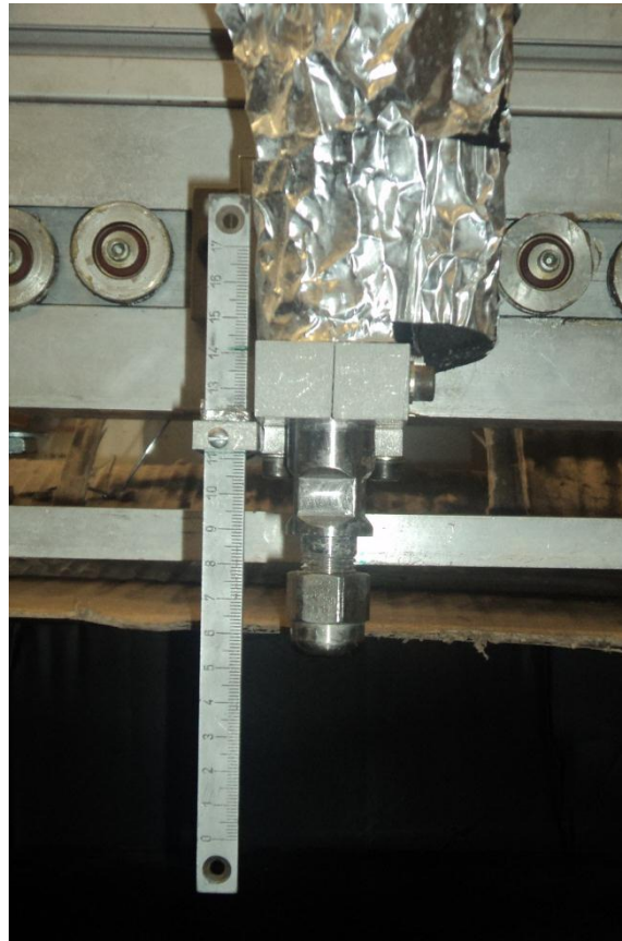
Figure 36: Image calibration system.
