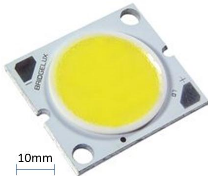
Figure 31: One of two high power LED diodes used for illumination of the jet.
