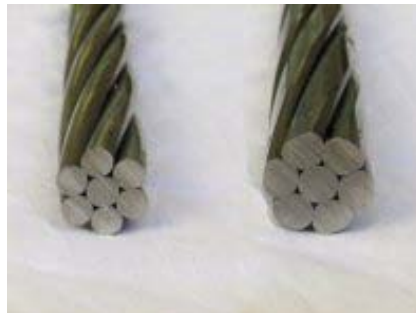
Figure 3.7 seven wire strands: wound and drawn.
