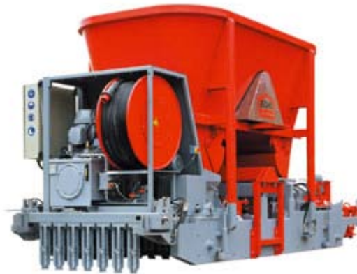
Figure 3.11 Top to bottom: extruding machine (Elematic) and slipformer (Echo engineering)
