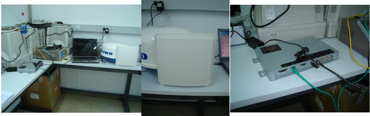
Figure 37. Fixed reader set up with 7 dBi antenna.
