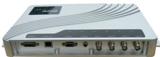
Figure 5. RFID 4 antennas Fixed Reader.
