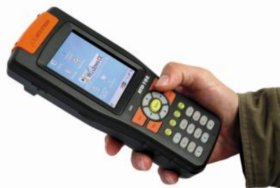
Figure 136. Aspect of the Marktrace RFID handheld reader selected for deployment of the pilot at the sea-platform.
