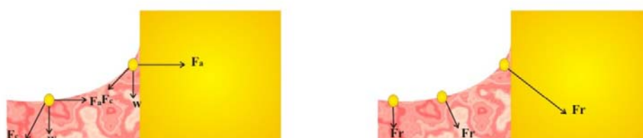
Fig 4.13 Receding meniscus effect In the left sketch it is shown how the forces are exerted in two gold nanocolloids. In the right sketch the resultant forces can be observed. When the molecules are far away from the wall, the resultant forces due to the weight and to the cohesion forces are vertical (the adhesion forces in this case are negligible), therefore the surface will be horizontal instead of vertical [6]
