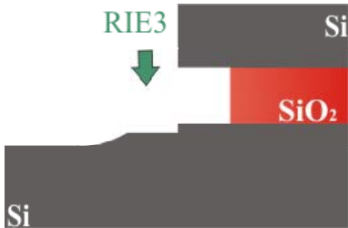
Fig 3.6 Third RIE step. This sketch shows us the result in the geometry of the devices after applying the RIE3, we remove the geometrical displacement between the upper and the lower electrode and a more symmetrical geometry it is achieved.
