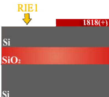
Fig 3.2 First RIE step This sketch shows us the application zone of the RIE1, as well the positive 1818 photoresist that is placed on the first silicon layer, after the a lithography step.
