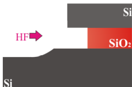
Fig 3.5 Selective nanogap etching step This sketch shows the formation of a trench by the selective removing of the silicon oxide with HF.
