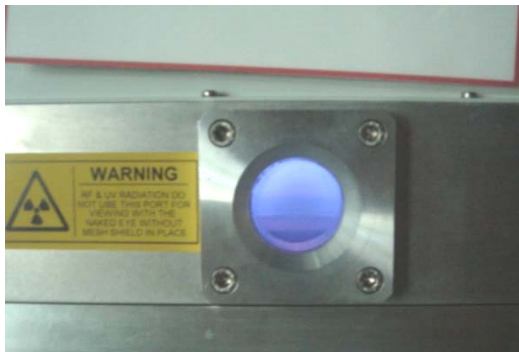
Fig 2.13 Detail in the plasma chamber. The plasma generated can be observed through the window.
