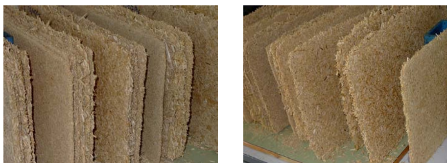
Figure 2. Wood-reed boards (left dry particles, right humid particles)
