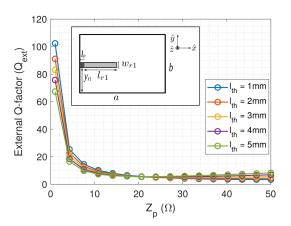
**FIGURE 5.** External quality factor  $Q_{ext}$  as a function of the input port reference impedance  $Z_p$ , for various values of the bar thickness  $l_{th}$ . The test frequency is  $f_c = 3.5$  GHz. Other dimensions are:  $I_d = 10$  mm,  $I_a = 10$  mm,  $y_{r1} = 10$  mm,  $w_{r1} = 2$  mm, a = 38 mm, b = 32 mm. The dark area  $I_p$  denotes a lumped port that models the direct connection of the coaxial pin to the resonator.
