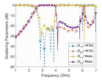
FIGURE 15. Comparison between the S-parameters simulated using the full-wave commercial software HFSS and measured data from the manufactured prototype shown in Fig. 13 (out of band performance).
