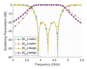
**FIGURE 8.** Scattering parameters of the in-line filter obtained with HFSS (design) and compared to the coupling matrix response (matrix). The bandwidth is  $BW_1 = 800$  MHz ( $FBW_1 = 18.78\%$ ). The dimensions are reported in Table 1.
