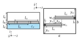
**FIGURE 3.** Side (left panel) and top (right panel) view of two coupled thick bar resonators, showing relevant dimensions. Feeding ports are shown with dark areas  $I_p$ .
