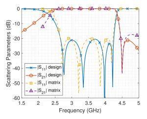
**FIGURE 11.** Scattering parameters of the third designed filter obtained with HFSS (design) and comparison to the coupling matrix response (matrix). The bandwidth is  $BW_3 = 1.57$  GHz ( $FBW_3 = 47.01\%$ ). The dimensions of this third design are reported in the third column of Table 2.
