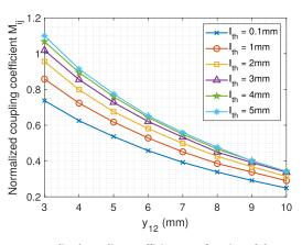
**FIGURE 4.** Normalized coupling coefficient as a function of the separation between resonators  $y_{12}$ , for various bar thicknesses  $l_{th}$ . Coupling coefficient is normalized with the first frequency plan ( $f_{c2} = 3.26$  GHz,  $BW_2 = 1.15$  GHz,  $FBW_2 = 35.28\%$ ). Other dimensions are: a = 30 mm, b = 28 mm,  $y_{r1} = y_{r2} = 10$  mm,  $w_{r1} = w_{r2} = 2$  mm,  $x_{12} = 0$  mm,  $l_d = 10$  mm,  $l_g = 10$  mm,  $e_r = 2.1$ .
