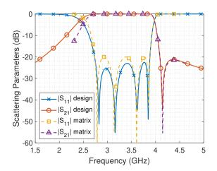
**FIGURE 10.** Scattering parameters of the second designed filter obtained with HFSS (design) and comparison to the coupling matrix response (matrix). The bandwidth is  $BW_2 = 1.15$  GHz ( $FBW_2 = 35.28\%$ ). The dimensions of this second design are reported in the second column of Table 2.
