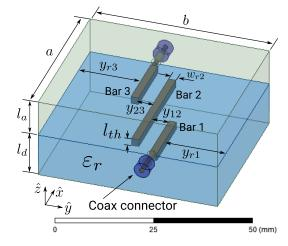
**FIGURE 1.** 3D view of the proposed filter technology based on bulky bars buried in a dielectric medium. The sketch shows an example of a filter using three bar resonators enclosed in a house cavity. I/O couplings are implemented with the step impedance discontinuity produced from a direct connection of the coaxial connectors with the first/last bar resonators.
