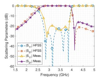
FIGURE 14. Comparison between the S-parameters simulated using the full-wave commercial software HFSS and measured data from the manufactured prototype shown in Fig. 13.
