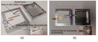
FIGURE 13. Manufactured prototype. (a) Components of the filter before assembling, and details of the slots in the Teflon substrate used for alignment. The inset inside shows the step discontinuity needed in the radius of the outer conductor for the I/O coupling adjustment. (b) Top view of the structure after assembling. Inset shows details of the assembling process between the coax center pin and the copper bar.
