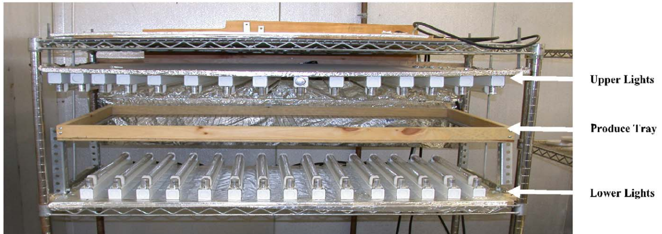
Fig. 1. UV-C radiation device. The arrows indicate the upper and lower groups of UV-C lights and the produce tray consisting of a polystyrene net and wooden frame.
