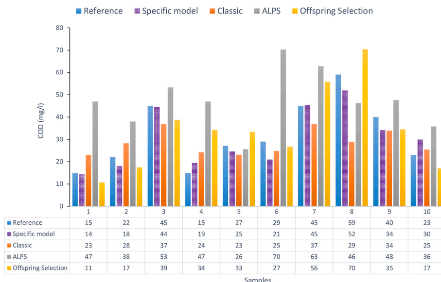
Fig. 6. Comparison of estimation between combined models and specific model for COD calculation.
