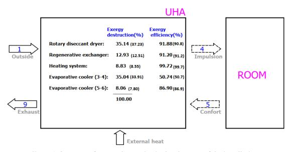
Figure 8. Summary of exergy destruction in the elements of the installation.
