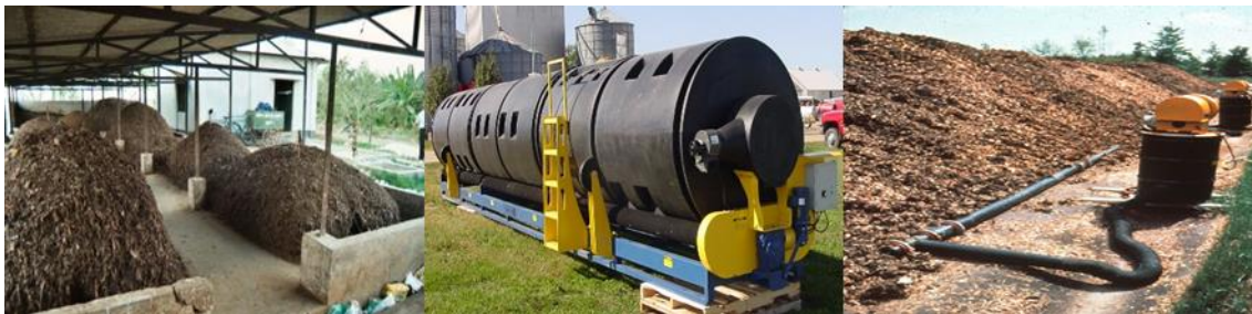
Image 10. Windrow composting, In-vessel composting, Aerated static pile
