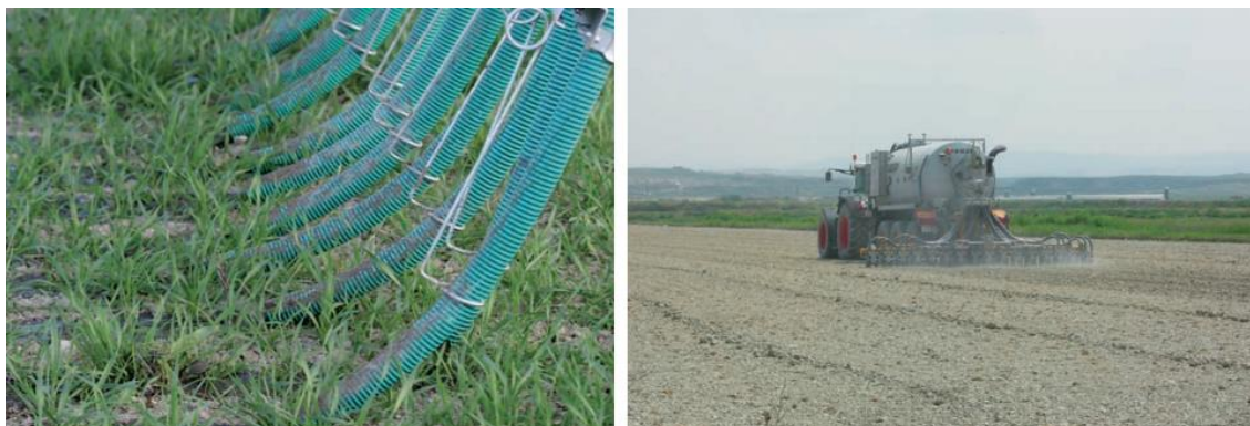
Image 1. Application systems of Pig manure with hoses and discs
