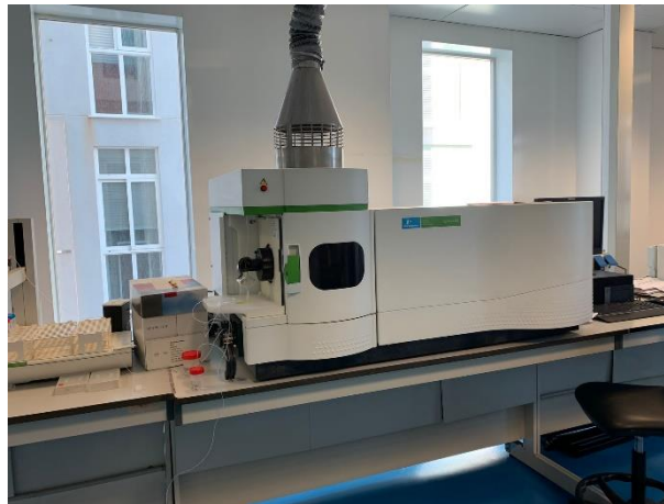
Photo 23. Coupled plasma mass spectrometry (ICP-MS), using Agilent 7900 (Perkin Elmer AA-Analyst 800)
