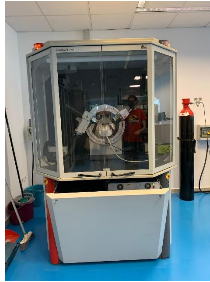
Photo 24. Bruker D8 Advance X-ray Diffractometer (XRD)
