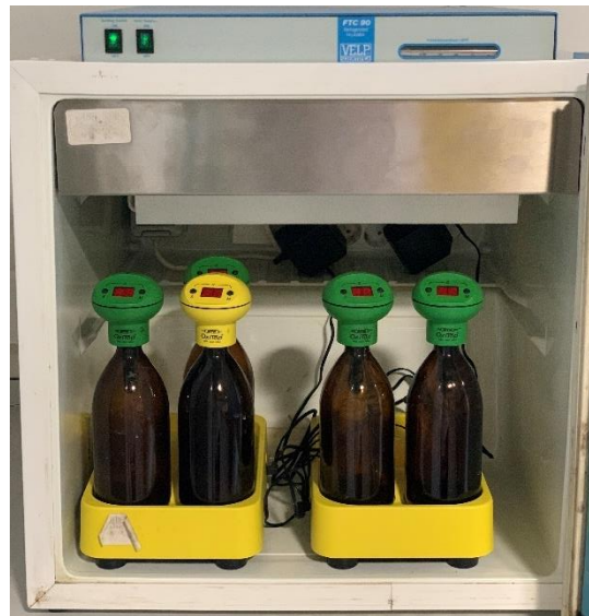
Photo 15. OXITOP BOD Instrumentation
