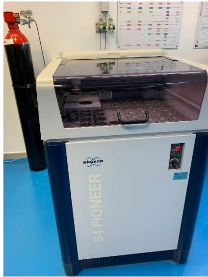
Photo 25. Bruker S4 Pioneer (XRF) spectrometer
