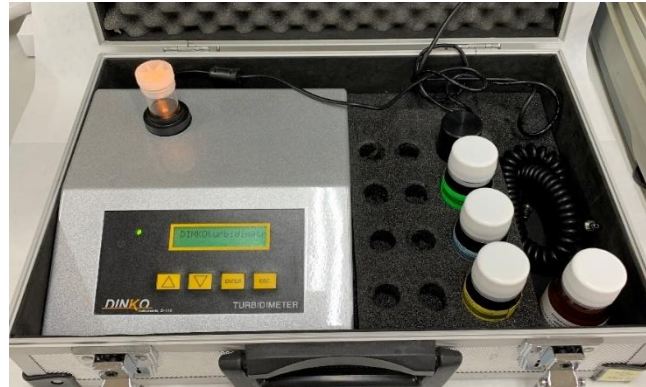
Photo 13. DINKO Turbidimeter D-110IR
