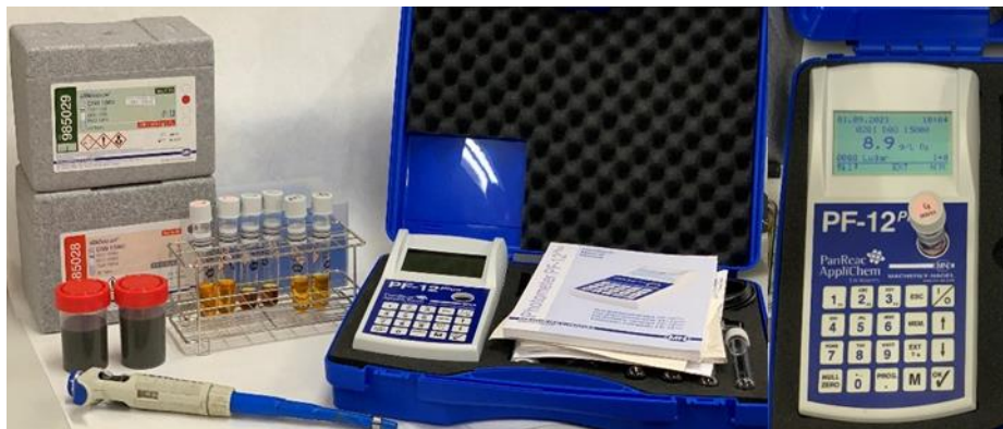
Photo 14. COD analysis equipment with Photometer NANOCOLOR PF-12
