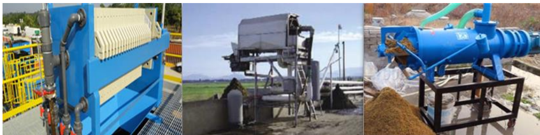
Image 4. Filter Press, Screw press, Roller press
