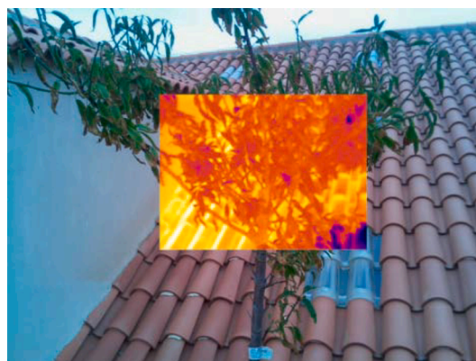
Fig. 4. Example of sensor image cropping to match FLIR SC305 field of view. Example of FLIR SC305 thermal image overlay on sensor visible image.
