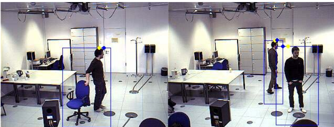
Figure 4.1.4. illustrates the behavioral features of the Background Subtraction method.
