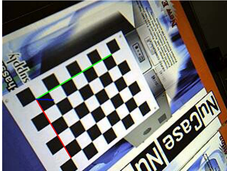
Figure 2.5.2. chessboard-reference-frame, (red \rightarrow x-axis, green \rightarrow y-axis, blue \rightarrow z-axis)
