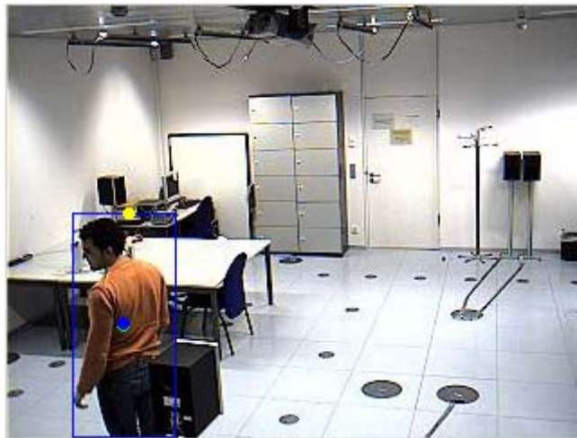
Figure 3.4.1. Person tracked with method based in differencing frames background subtraction combined with a Kalman Filter. The blue box represents the region belonging to the foreground.
