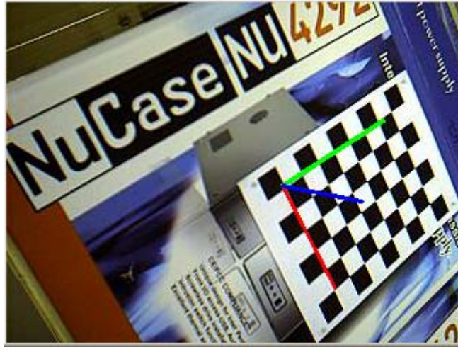
Figure C.2. shows the projection of the computed reference-frame.
