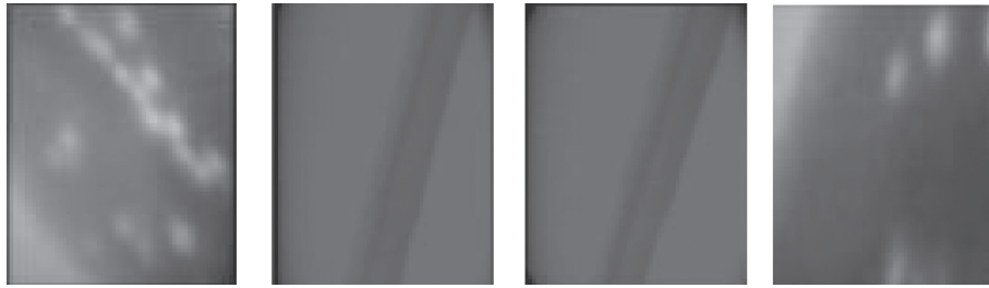
FIGURE 9: Results of application of DCFA (from left to right): porosities defects image classified as follows: lack of penetration defect image, well-classified lack of penetration defect image, well-classified lack of penetration defect image, and well-classified porosities defects image.
