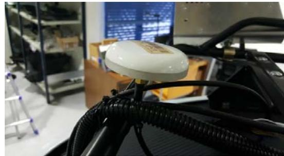
Figura 17. Antena GPS 2G15A-XS-1
