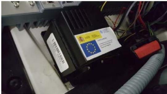
Figura 16. IMU Moog Crossbow NAV440CA-202
