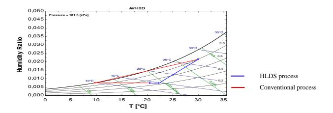
Figure 6: Air treatment processes in the HLDS and in a conventional cooling system.
