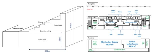
Figure 2. Location and distribution of the locker rooms of Taiwan Building Technology Center in Taipei
