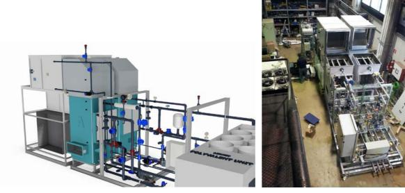
Figure 7:3D CAD design and prototype of the HLDS in the laboratory
