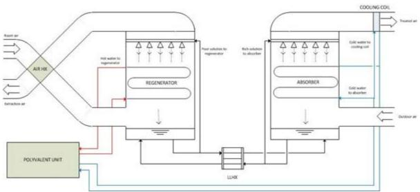
Figure 1.Hybrid liquid desiccant cooling system.
