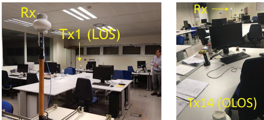
Figure 5. View of the Rx antenna and the Tx antenna in positions Tx1 in LOS (left) and Tx14 in OLOS (right).
