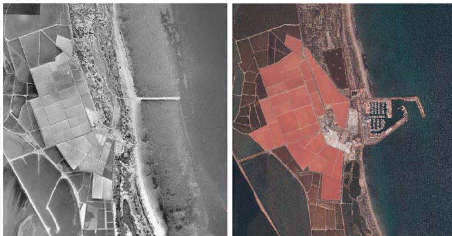
Fig. 6. San Pedro del Pinatar marina's impact on the sand line in south-eastern Spain.
