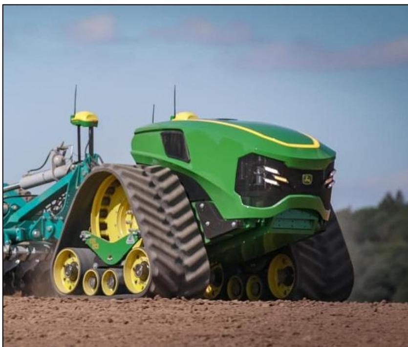
Figura 1. Tractor autónomo John Deere.
