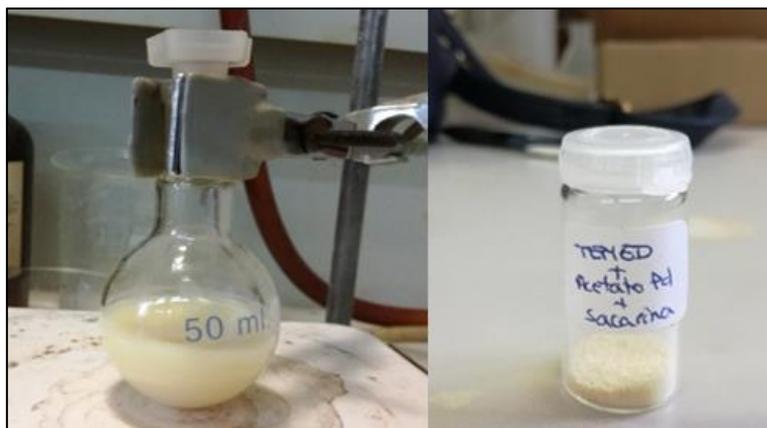
Figura 3.8.  $[\text{Pd}(\text{tmeda})(\text{sac})_2]$ .
