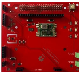
Figura 19. LoRaWAN Gateway Backplane.
