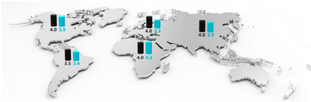
Fig. 5. Equivalent inertia constants estimated in the world by continent. Change between 1996 and 2016.
