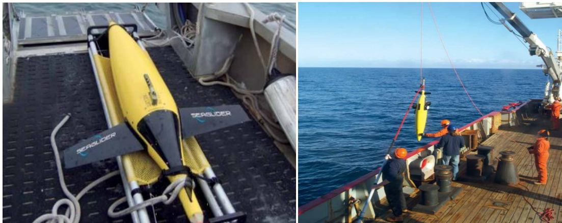
Fig.2.6. Launching methods for Seagliders (Source: [38])
