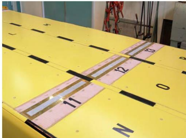
Figure 1.9: Bottom configuration for micro bubbles where porous strips were placed to allow air bubble flow.
