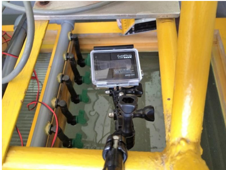
Figure 2.14: GoPro mounted on carriage structure.
