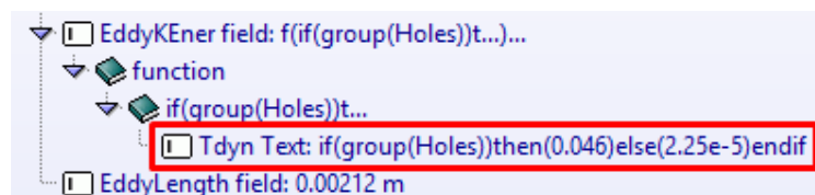
Figure 3.31: Conditional function for establishing the Eddy Kinetic Energy in the holes and in the mixture for the Spalart Allmaras turbulence model.
