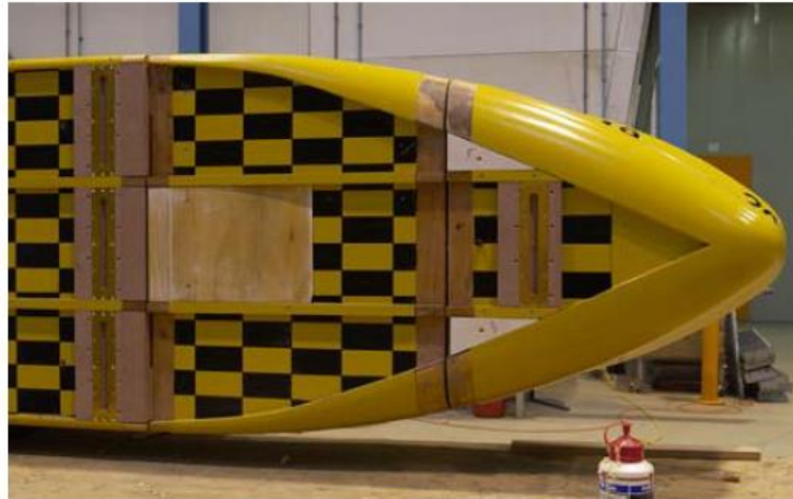
Figure 1.10: Detail of bottom configuration of segmented ship model during preparations.
