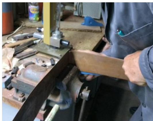
Fig. 2.20: Bending side plates.
