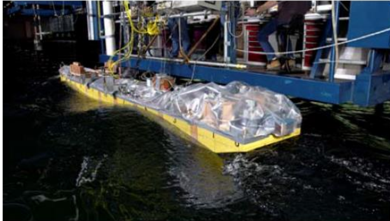
Figure 1.12: Model testing in waves.
