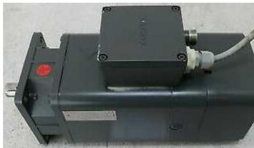
Figura 3-11: Servomotor 1FT5074
