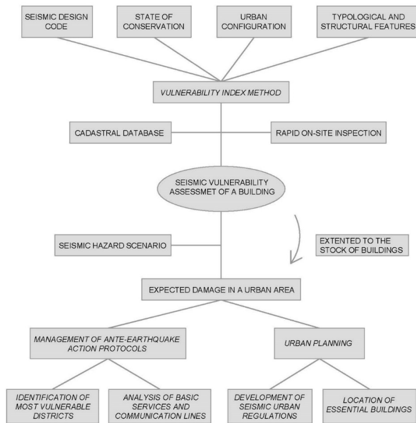
Figure 10. Diagram of the implementation of the proposed model of the LM1 method applied to the planning and management of ante-earthquake emergency scenarios. The issues developed in this contribution are italicized.
