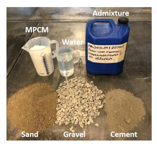
Figure III.4. Ingredients of Portland cement concrete mixture.
