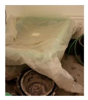
Figure III.8. Curing samples in water at 40 °C.
