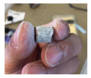
Figure III.19. Sample preparation for X-ray tomography imaging.
