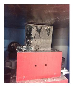
Figure III.16. A failed GPC sample after compressive strength test.
