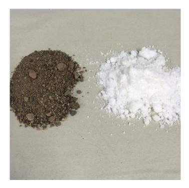
Figure III.2. Illustrative picture of sand and MPCM for replacement method.
