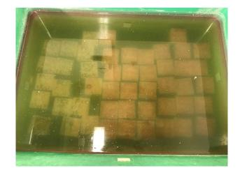
Figure III.7. Curing samples in water at 20 °C.
