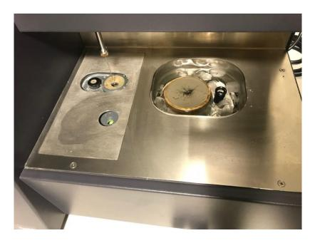
Figure III.10. Setting time measurement at 0 °C.
