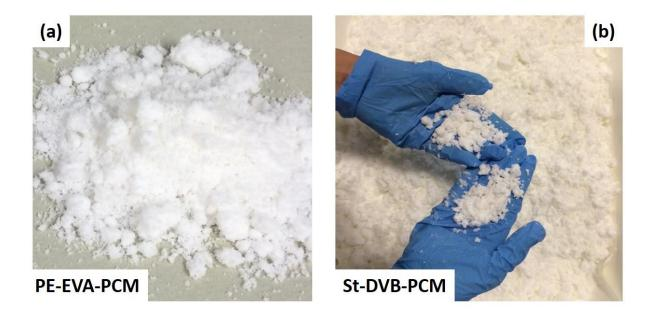
Figure III.1. Illustrative pictures of the appearance of (a) PE-EVA-PCM, (b) St-DVB-PCM.
