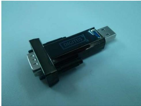
Figura 2.10: conector rs232-usb
