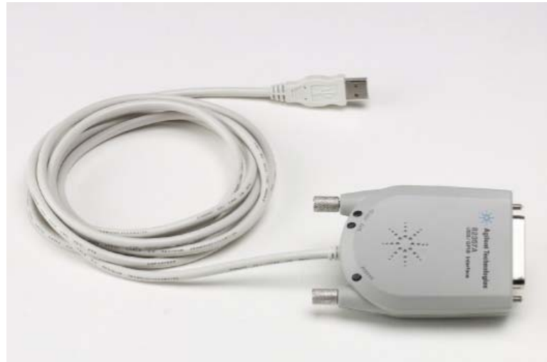
Figura 9- Cable GPIB-USB Agilent 82357A
