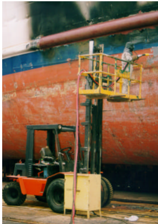
Fig. 1. Present method for hull cleaning
