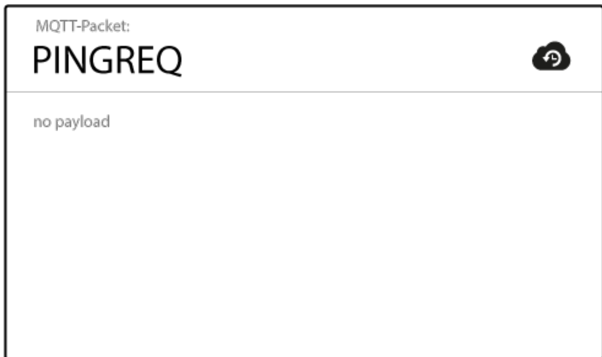
Figure 4.15: PINGREQ packet structure
