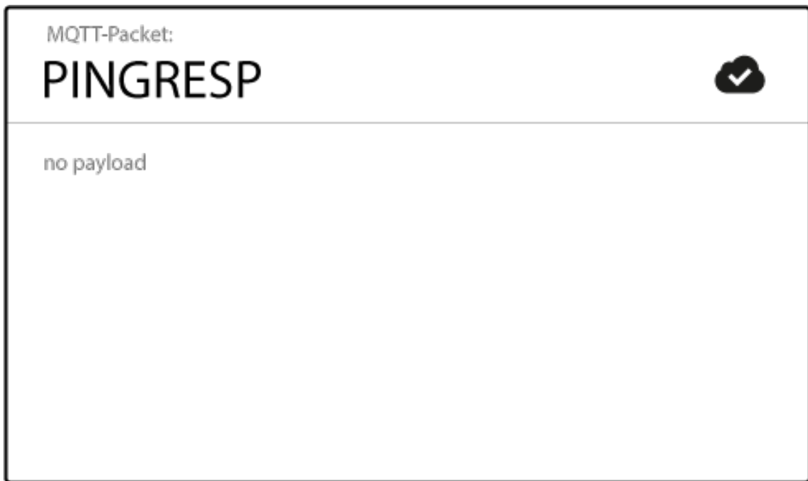
Figure 4.16: PINGRESP packet structure
