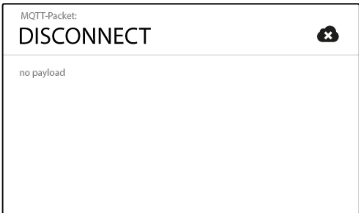
Figure 4.17: DISCONNECT packet structure
