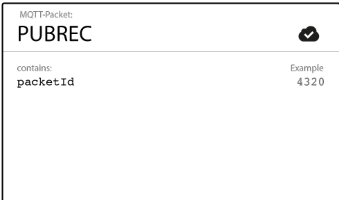
Figure 4.8: PUBREC packet structure
