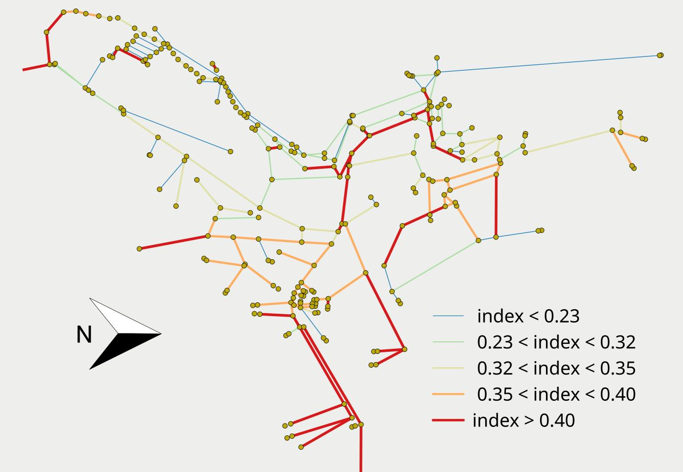
Figure 2: Pipe categorisation attending to the weighted index from the pipes in which a leakage would lead to worse effects (greater index), to the pipes with less important effects (fewer index).
