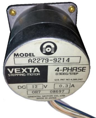
Figura 3.16: Motor PAP VEXTA A2279-9214
