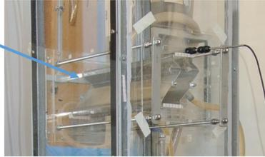
An experimental prototype of a mechanical draft cooling tower has been set up to study the interaction of air and water in a drift eliminator. It consists on a prismatic structure; an airstream is introduced from the bottom of the tower; and a water circuit injects water inside the tower, through one of the plates of the drift eliminator, forming a water film simulating the films formed by the atomization of water in real towers.
