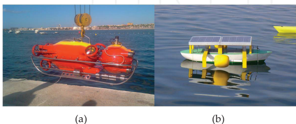
Figure 3. Test of navigation on the Mar Menor lagoon. (a) Underwater Submarine. (b) Surface boat.
